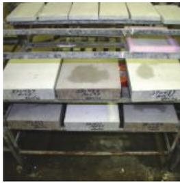
ASTM C 779 abrasion testing device.
