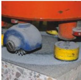
Concrete specimen after abrasion testing.
