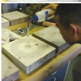
Rilem Tube filled with water. (close up view)
